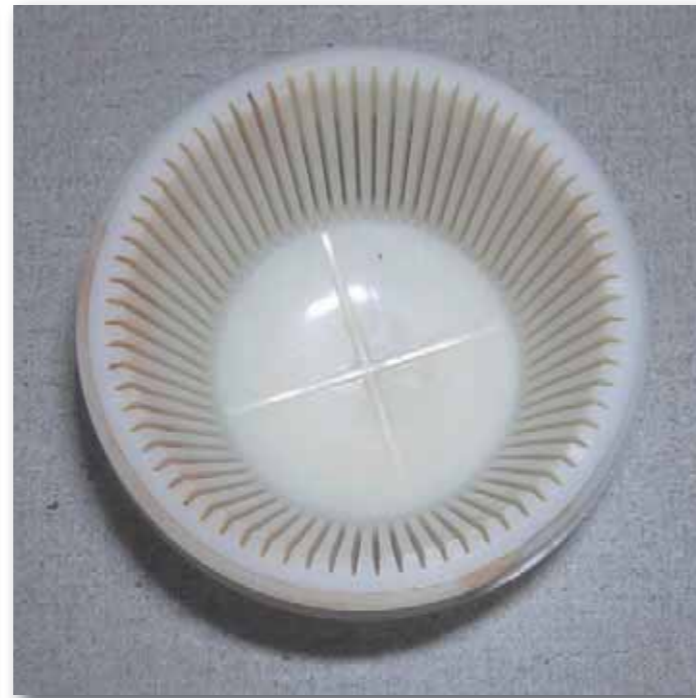
After treatment, microscopy performed on the filter samples at Ashford showed that visible deposits had been removed and the media successfully restored to a near-new condition
